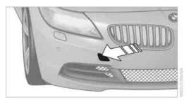
Release the cover panel in the bumper: Press on the recess at the bottom left in the cover panel.
