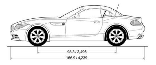
All dimensions given in inches/mm. Smallest turning circle diam.: 36 ft 1 in/11.0 m.
