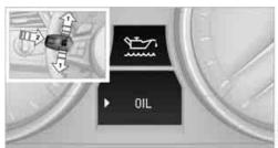
Press button 1 in the turn indicator lever up or down repeatedly until the appropriate symbol is shown in the display, accompanied by the word "OIL".
