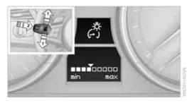
Press button 1 up or down to select the desired brightness level.
