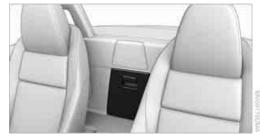
In the cargo bay: press the tab up and fold the cover down.
