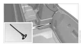
Pull the button in the cargo bay with the fuel pump symbol down. The fuel filler door is released.
