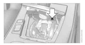
Using the screwdriver from the onboard tool kit, refer to page 208, press the red lever while moving the selector lever to the desired position.
