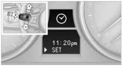
Press button 1 in the turn indicator lever up or down repeatedly until the appropriate symbol appears in the display, accompanied by the time and the word "SET".
