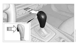
A lock prevents you from inadvertently engaging selector lever positions R and P. To cancel the lock, press the button on the front of the selector lever, see arrow.
