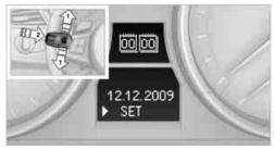
Press button 1 in the turn indicator lever up or down repeatedly until the appropriate symbol appears in the display, accompanied by the date and the word "SET".
