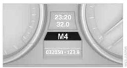
P, R, N, D1 to D7, S1 to S7, M1 to M7 The transmission position and the gear currently engaged are displayed.
