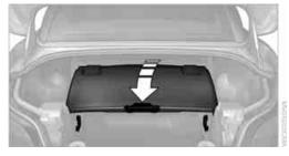
Before opening the hardtop, close the cargo bay partition, arrow, and make sure it engages on both sides.
