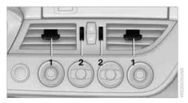
1 Use the lever to change the direction of the air flow
