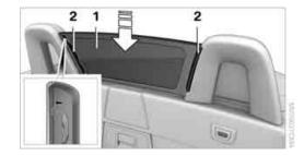
Push the wind deflector down, arrow 1, and then push down and forward simultaneously, arrow 2, until it engages.
