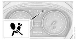
As of radio readiness, refer to page 50, the warning lamp comes on briefly to indicate that the entire airbag system and the belt tensioners are operational.
