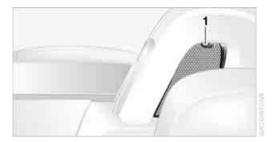
Clothes hooks **1** are located on the wind deflector panels in the rollover bars.
