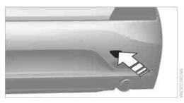
Release the cover panel in the bumper: Press on the recess at the bottom center in the cover panel.
