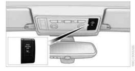
The indicator lamp for the passenger airbags shows the functional status of the passenger's front, knee and side airbags in accordance with whether and how the passenger seat is occupied. The indicator lamp shows whether the passenger airbags are activated or deactivated.
