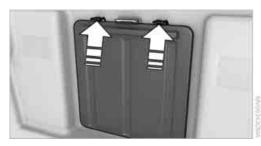
In the cargo bay: Press the handle up and fold the transport bag completely down.
