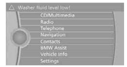
Text messages at the upper edge of the Control Display explain the meaning of the displayed indicator and warning lamps.
