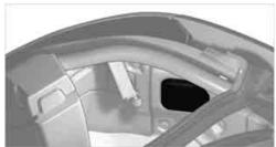
2. Pull out the bulb holder, see arrow, and change the bulb.
