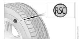
The symbol identifying Run-Flat Tires is a circle with the letters RSC on the sidewall. Run-Flat Tires comprise a conditionally selfsupporting tire and a special rim. The reinforcement in the sidewalls ensures that the tire can continue to be used subject to certain restrictions, even if depressurized.
