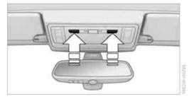
The reading lamps are located next to the interior lamps. To switch on and off, press the button.
