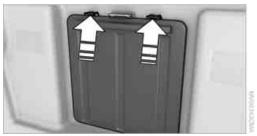
In the cargo bay: Press the handle up and fold the storage compartment completely down.
