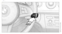
Inserting the remote control all the way into the ignition lock.
