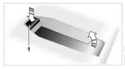
2. Insert the snap-in adapter at the front and press it downward until it engages.
