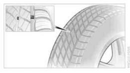
Wear indicators in the base of the tread groove are distributed around the tire's circumference; the letters TWI, for Tread Wear Indicator, on the tire's sidewalls identify tires that incorporate these wear indicators. Once the tire tread has worn down to the wear indicators, the tire has worn to a depth of 1/16 in/1.6 mm.
