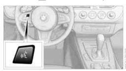
This symbol on the Control Display and an acoustic signal indicate that the voice activation system is ready to receive spoken commands.
