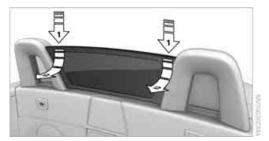
The wind deflector must engage firmly, otherwise it could become detached at higher vehicle speeds. ◀
