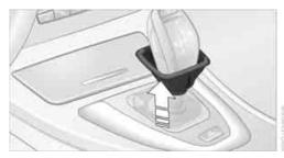
3. Remove the cap using the Allen wrench from the onboard tool kit, refer to page 208.
