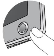
Turn on the monitor by pressing the power button on the right of the monitor.
