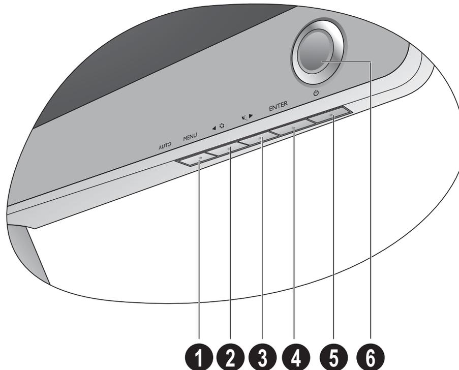
1. **AUTO**: Adjusts vertical position, phase, horizontal position and pixel clock automatically.
