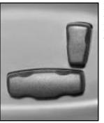
If you have this feature, the power seat controls are located on the outboard side of the front seat cushions.
