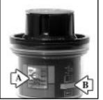
The engine air cleaner/filter assembly has an indicator that lets you know when the air filter is dirty and needs to be serviced. The indicator is located on the engine air cleaner/filter air duct.
