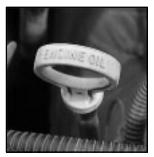
The engine oil dipstick handle is a yellow ring located in the engine compartment toward the passenger's side of the vehicle. See "Engine Compartment Overview" in the Index for more information on location. Turn off the engine and give the oil several minutes to drain back into the oil pan. If you don't, the oil dipstick might not show the actual level.
