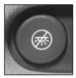
You can use the dome override button, located below the exterior lamps knob, to set the dome lamps to come on automatically when a door is opened, or to remain off. To turn the lamps off press the button. The dome lamps will remain off when a door is open. To return the lamps to automatic operation, press the button again. The dome lamps will come on when you open a door. This will override the illuminated entry feature unless you use your keyless entry transmitter to unlock the vehicle.
