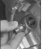
9. Put the nuts on by hand. Make sure the rounded end is toward the wheel.
