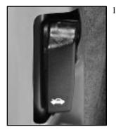
1. To open the hood, first pull the handle located inside the vehicle on the lower driver's side of the instrument panel.
