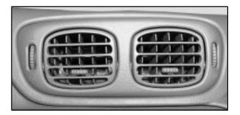
Your vehicle has air outlets that allow you to adjust the direction and amount of airflow inside the vehicle. Move the louvers up or down and move the control in the center of each outlet side-to-side to direct the air from the outlet. Use the thumbwheel next to or underneath the outlet to close the louvers. For the most efficient airflow and temperature control, keep the outlet in the fully opened position.
