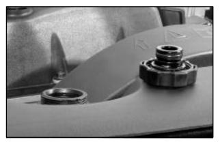
2. Then keep turning the pressure cap. Remove the pressure cap.
