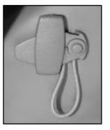
1. Slide the guide off of its storage clip located between the interior body and the seatback.
