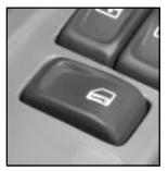
The power door lock switches are located on the driver's and front passenger's armrests.
