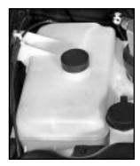
When the engine is cold, the coolant level should be at least up to the FULL COLD mark. If it isn't, you may have a leak in the radiator hoses, heater hoses, radiator, water pump or somewhere else in the cooling system.
