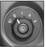
This control is located to the right of the steering wheel on the instrument panel.
