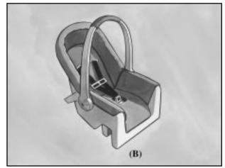
An infant car bed (A), a special bed made for use in a motor vehicle, is an infant restraint system designed to restrain or position a child on a continuous flat surface. Make sure that the infant's head rests toward the center of the vehicle. A rear-facing infant seat (B) provides restraint with the seating surface against the back of the infant. The harness system holds the infant in place and, in a crash, acts to keep the infant positioned in the restraint.
