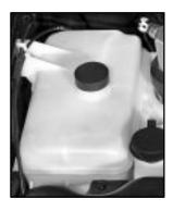
The engine coolant recovery tank is in the engine compartment on the passenger's side of the vehicle. See "Engine Compartment Overview" in the Index for more information on location.
