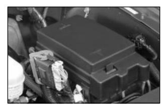
The fuse block is located under the hood in the engine compartment on the driver's side of the vehicle. See "Engine Compartment Overview" in the Index for more information on location.
