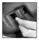
You should adjust the steering wheel before you drive. The tilt lever is located on the driver's side of the steering column, under the turn signal lever.
