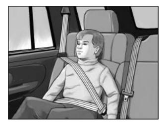
4. Buckle, position and release the safety belt as described in "Rear Seat Passenger Positions" earlier in this section. Make sure that the shoulder belt crosses the shoulder.
