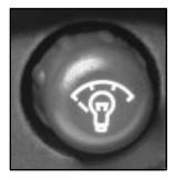
Press the knob located next to the exterior lamps knob to extend and turn it to make your instrument panel lights brighter. Turn the knob all the way up to turn on the interior lamps. Press the knob back into its stored position.
