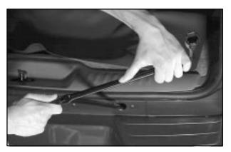
1. To remove the underbody-mounted spare, insert the socket end of the extension, on an angle, into the hole in the rear bumper. Be sure the socket end of the extension connects into the hoist shaft.
