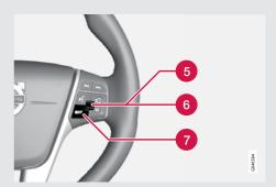
\* FAV - used to store frequently used functions, making it possible to start the stored function by simply pressing this button. See the example under SENSUS INFOTAINMENT - NAVIGA-TION MODE.
