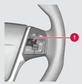
The voice control feature (only available in cars fitted with the optional navigation system) can be used to voice-activate certain functions on a Bluetooth®-enabled mobile phone and the navigation system.
