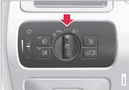
Light switch in position AUTO .
