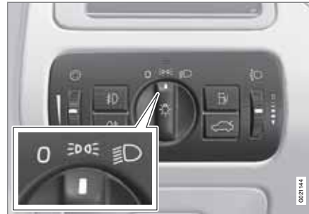
Headlamp control in position for position/parking lamps.
