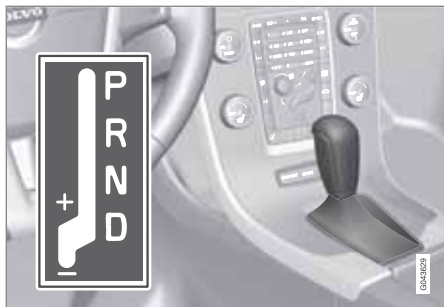
D: Automatic gear positions. +/-: Manual gear positions.
