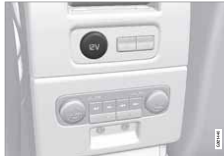
12 V socket in tunnel console, rear seat.
