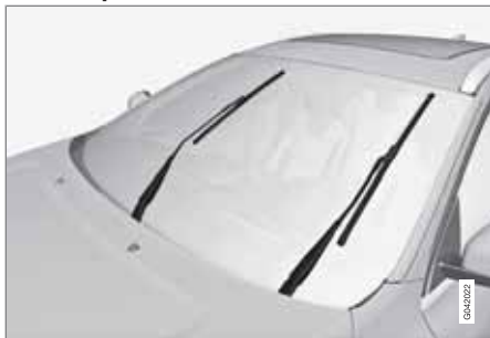
Wiper blades in service position.
