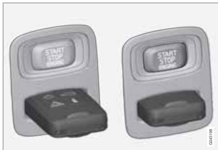
Ignition switch with remote control key extracted/inserted.
