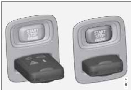
Ignition switch with remote control key extracted/inserted. and START/STOP ENGINE button.
