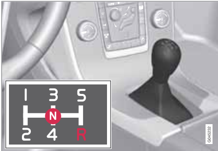
Gearshift pattern 5-speed gearbox.
