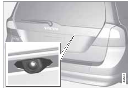
Camera location next to the opening handle.
