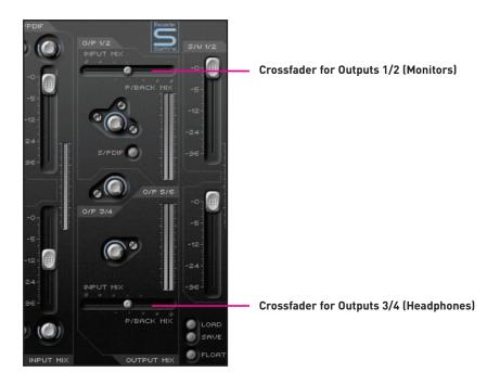
Setting either slider to the extreme right position will mean only Playback tracks will be heard on that stereo pair of Outputs. Then, moving the slider to the left will add increasing amounts of Inputs and decrease Playback tracks until, in the extreme left position, only Inputs are heard.
