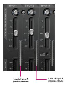
If recording a stereo signal then make sure that the Gain dials for both Inputs on the front of the hardware are set to the same level, observing the Input meters in the SaffireControl LE software, shown above.
