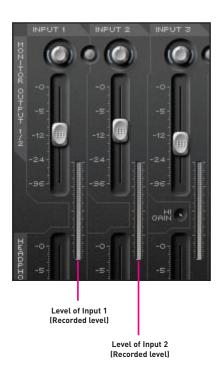
This signal will now appear as Saffire LE Input 1 or Input 2 (depending on which socket the microphone is connected to) within your sequencer/recording application.
