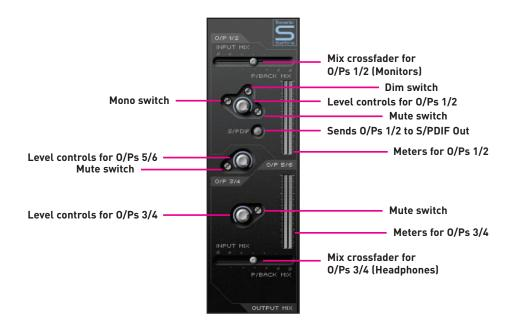
In addition to Mute switches, O/Ps 1/2 also offer a Mono switch for making the signal Mono, as well as a Dim switch for reducing the level by 12dB. If you want to send the O/Ps 1/2 signal to the S/PDIF Out for carrying out a digital transfer then the switch labelled S/PDIF, below the Gain dial for O/Ps 1/2, should be active.
