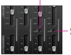
High Gain Switch for Input 4 – engage if an Instrument is connected
