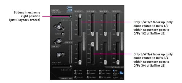
Similarly, although not visibly within the SaffireControl LE software GUI, only sequencer tracks routed to Saffre LE Outputs 5/6 and 7/8 will be sent to Outputs 5/6 (Analogue) and Outputs 7/8 (SPDIF), respectively.
