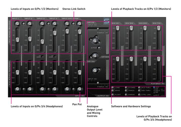
Each section of SaffireControl LE is explained in greater depth in relevant sections of the User Guide.
