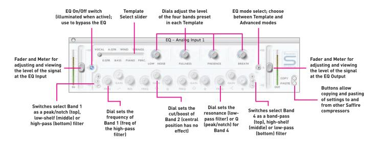
Equalisation of sound is an essential part of the recording process, necessary to remove or boost various sections of the audible frequency spectrum. The Saffire EQ is 4-band parametric, with the option of shelving and high/low-pass on bands 1 and 4, and exhibits the same curves as the classic Focusrite EQ; all that's required to sculpt sound with truly professional flair!
