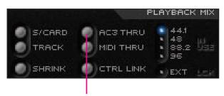
AC3 THRU switch – engage to stream AC3/DTS signal to S/PDIF Out
