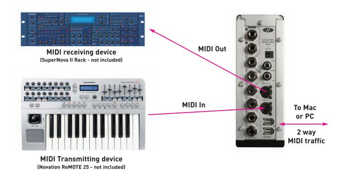
Saffire LE can operate in one of two possible MIDI modes. The state of the MIDI THRU switch in SaffireControl LE determines which MIDI mode will be used, as follows:
