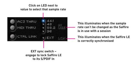
If wanting to synchronise to an external source (via the S/PDIF In signal), which is normally advisable when recording a S/PDIF signal, then press the EXT LED, which will illuminate once selected. Saffire LE will only be correctly synchronised to this source if LOK is illuminated next to it. If not, make sure that the sample rate of the incoming S/PDIF signal is the same as the one set in this window.
